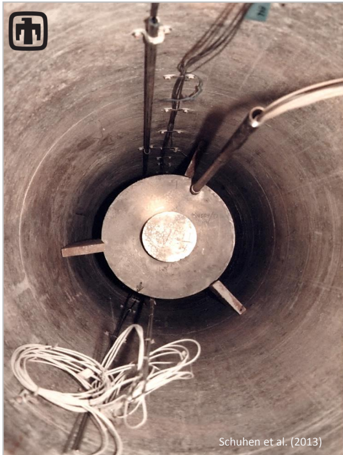
Typical WPP DHLW canister in Room B at installation and removal Creep closure and salt crust deposition required overcoring to remove
