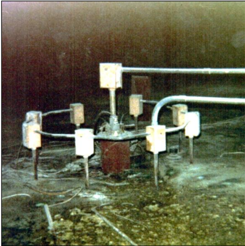
Figure 3. Avery Island Site C Test with 8 Guard Heaters
