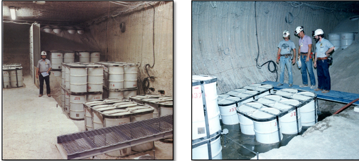
Figure 20. Room J CH TRU CH drums and crushed salt in brine pool experiment
