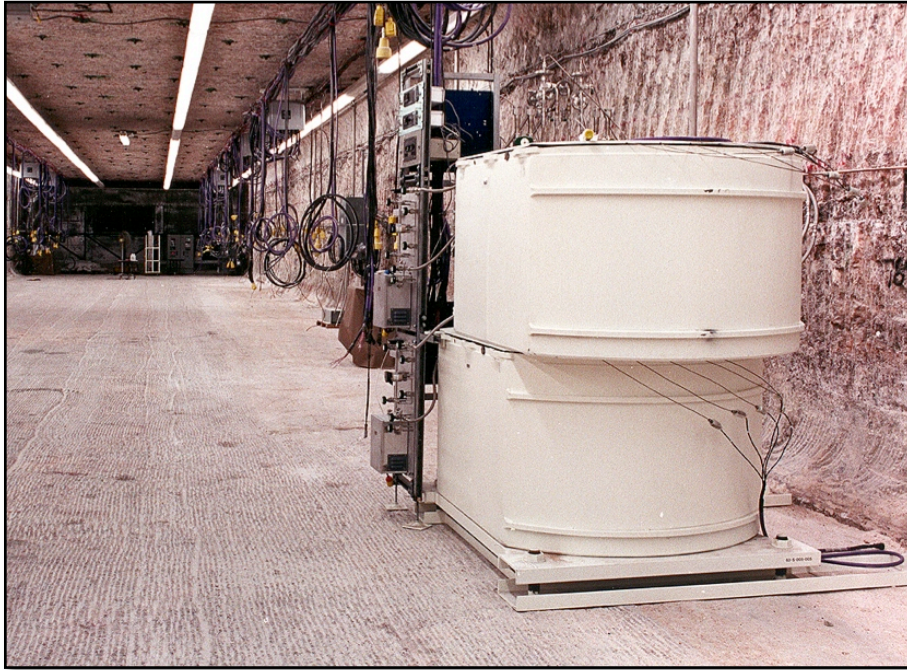
Figure 22. WIPP Bin-Scale Test instrumentation in alcove north of Panel 1
