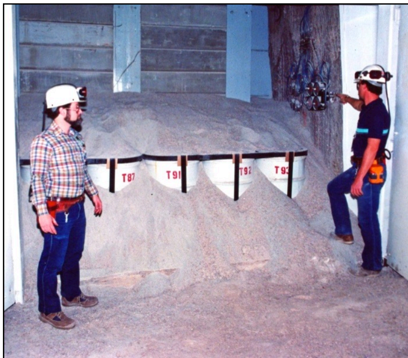
Figure 21. WIPP WPP Room T backfilled CH canister experiment
